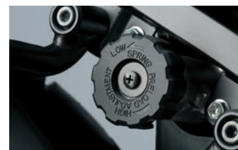
Useful spring preload adjustment
